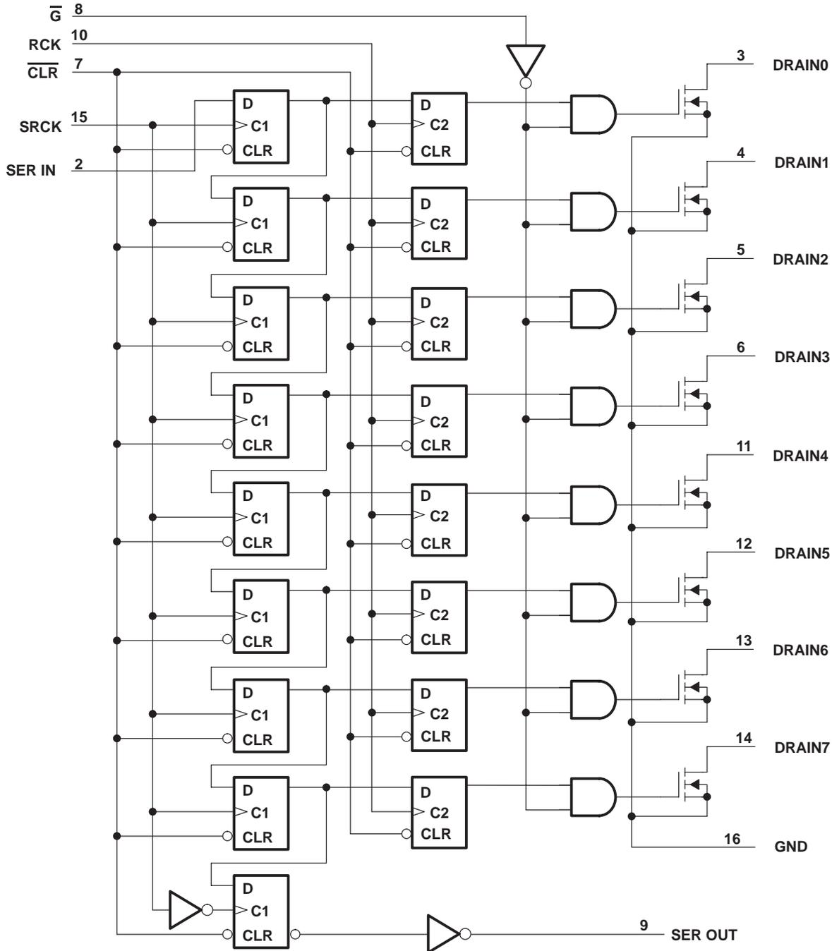
**schematic of inputs and outputs**
